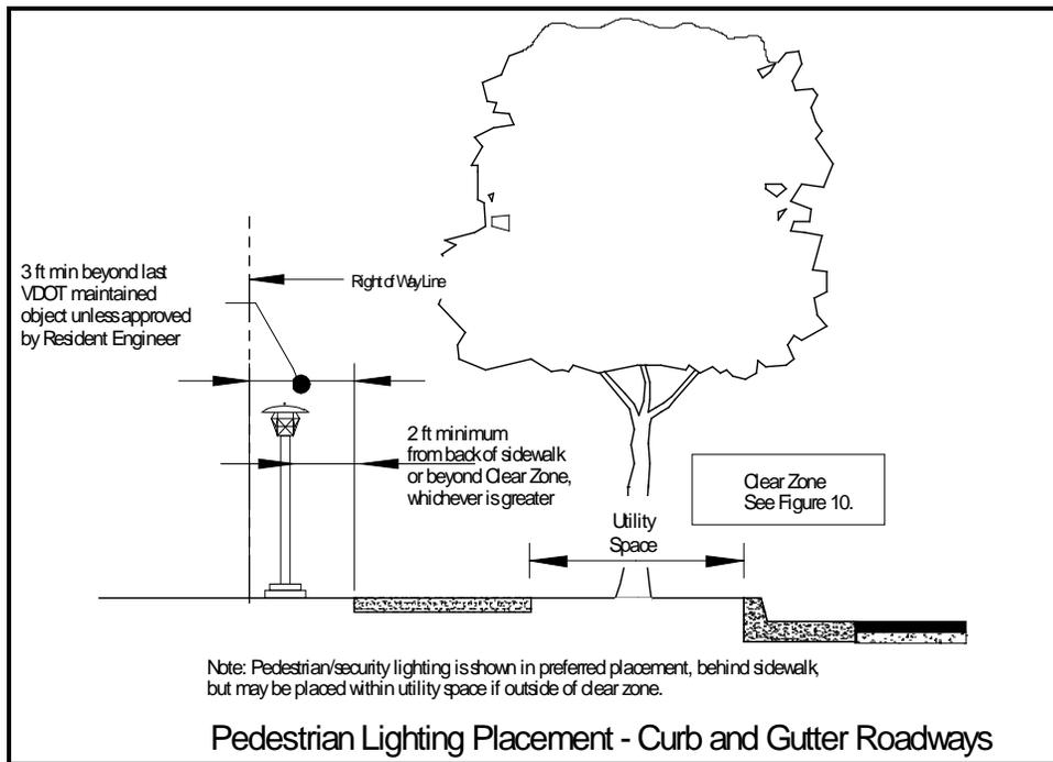
**FIGURE 13 – LIGHTING ALONG CURB AND GUTTER SECTIONS**
