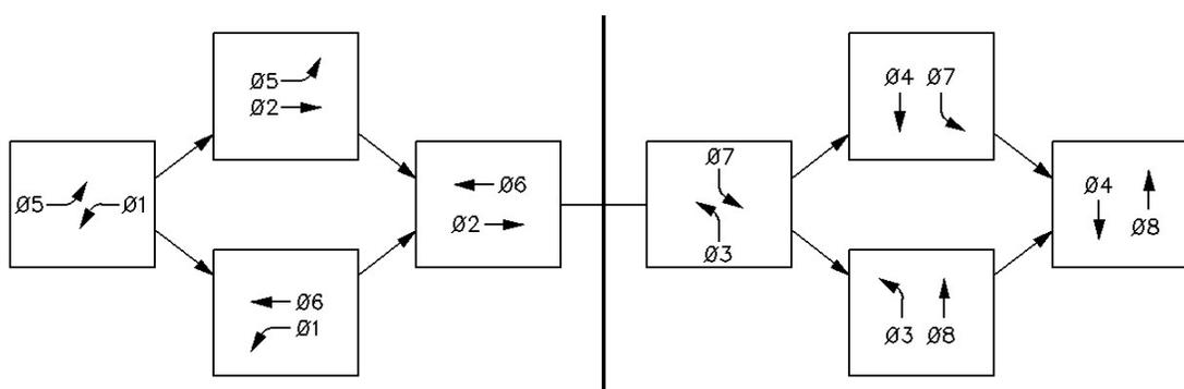
**Figure 2-5: BASIC PHASING COMBINATIONS FOR DUAL RING CONTROLLER**
