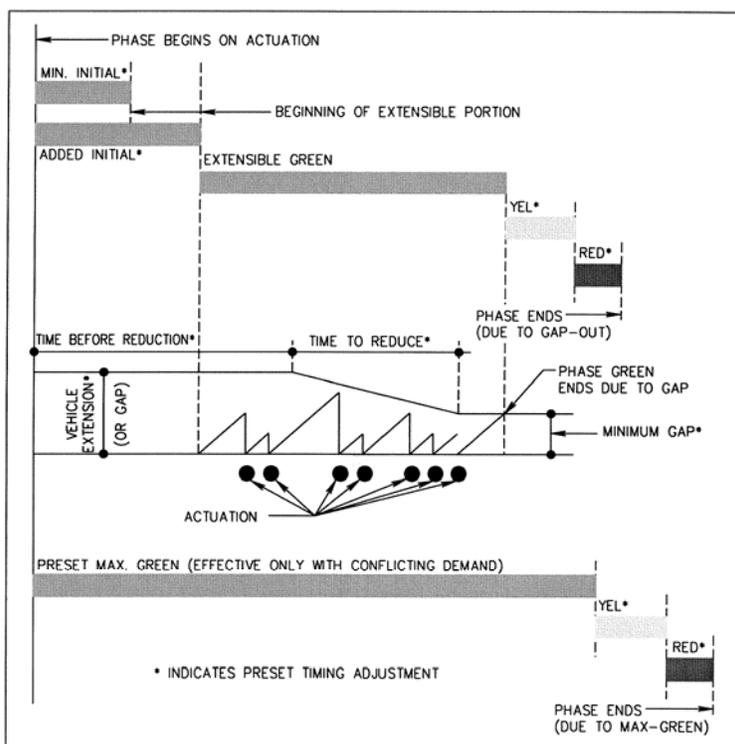
**Figure 2-6: SCHEMATIC DIAGRAM OF VOLUME-DENSITY CONTROL**
