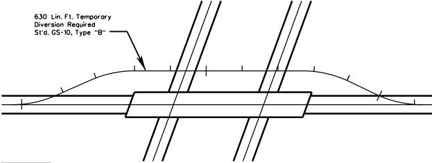
Diversions on crossroads carrying over 750 ADT should have the complete alignment, grades, typical sections, drainage, etc., shown on the plans. Additional temporary construction easement lines should also be shown, if necessary.
