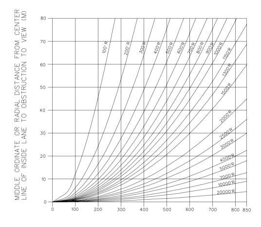
\* 0.5 FEET STOPPING 4.25 FEET PASSING LINE OF SIGHT AT MID POINT TO BE 2.0' ABOVE EDGE OF PAVE-MENT FOR STOPPING SIGHT DISTANCE, AND 4.0' FOR PASS-ING SIGHT DISTANCE.
