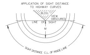
LENGTH OF ARC SUBTENDED OR CLEAR SIGHT DISTANCE MEASURED ALONG CENTER LINE OF INSIDE LANE (S)
