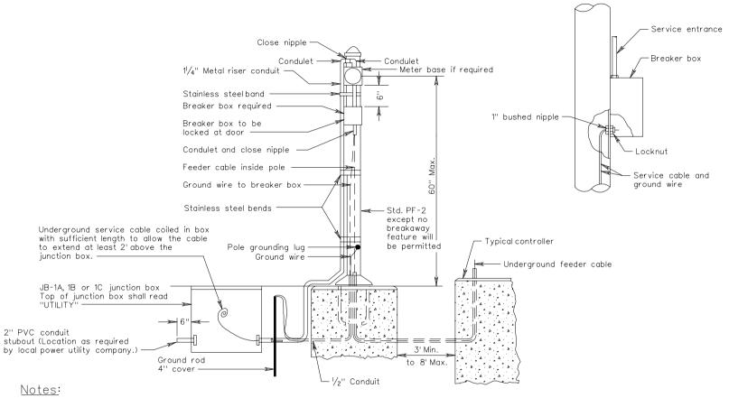
No other conductors shall be run in the same conduit with electrical service cable.
