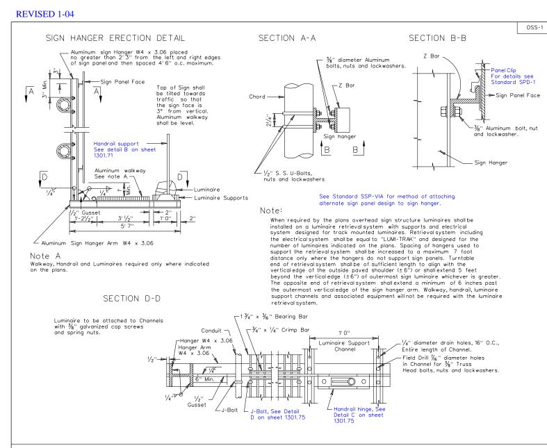
TYPICAL DETAILS FOR OVERHEAD SIGN STRUCTURES
