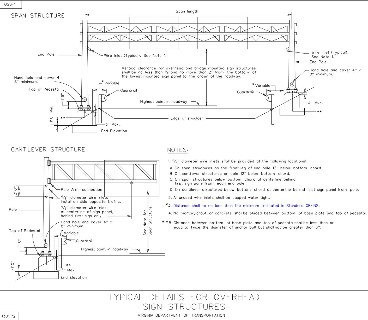
SIGN HANGER ERECTION DETAIL
