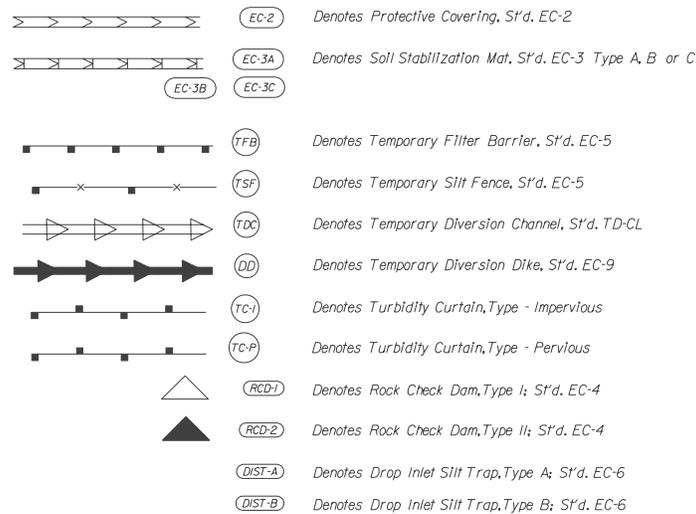
The ESC symbols are to be used to denote proposed erosion and sediment control items on the plans and are available in the CADD Cell and Custom Line Style Libraries and the GeoPak Road Plan View Labels.
